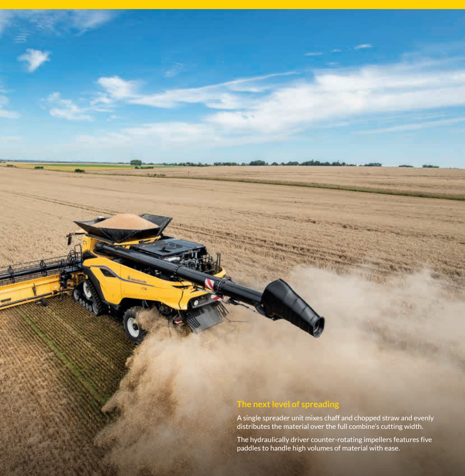
Chopping with grain configuration
